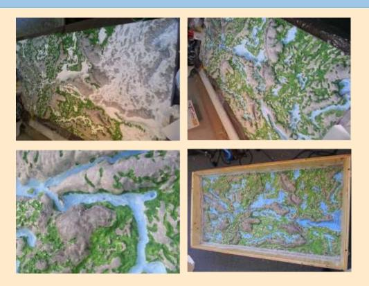
Photo 24: Clockwise from top left – Painting the grey, green and blue layers on the model. The complete model painted, inked and secured in the box.
