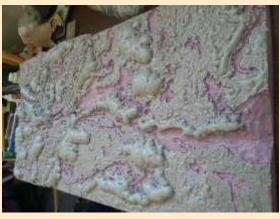
Photo 21: The second application of spray foam. This time the foam was spread around using scrap pieces of cardboard so that it would only expand a little. The image on the right is the end result.
