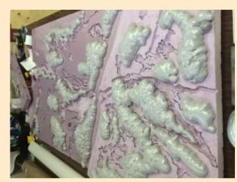
Photo 20: The first application of spray foam once it had fully expanded and cured.
